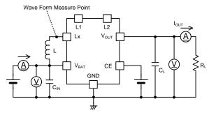
$\begin{aligned} & \times \text{External Components} \\ & \text{C}_{\text{IN}} : 10\,\mu\,\text{F( ceramic )} \\ & \text{C}_{\text{L}} : 10\,\mu\,\text{F( ceramic )} \\ & \text{L} : 1.5\,\mu\,\text{H(selected inductor)} \end{aligned}$
