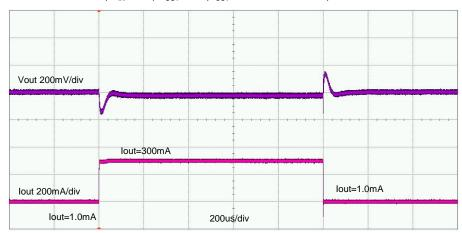
• XCL103D503CR-G,  $V_{IN}$ =3.7V,  $V_{OUT}$ =5.0V,  $I_{OUT}$ = 1.0mA  $\Leftrightarrow$  300mA , Ta=25°C
