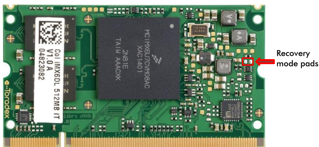
Figure 8 Location of recovery mode pads
