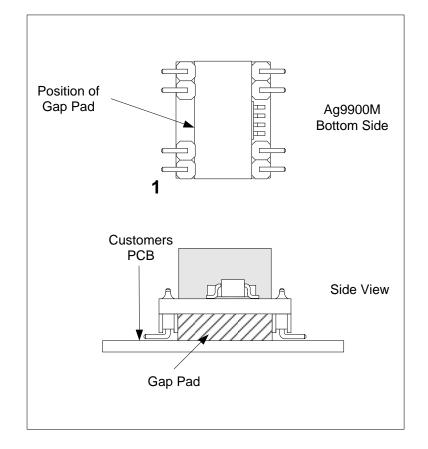
Figure 16: Thermal Gap Pad Position
