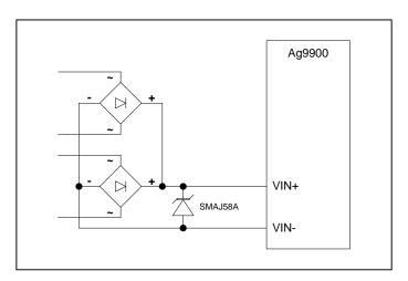
Figure 18: Ag9900 Input Protection
