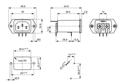
Screw and snap-in mounting with flexible wire
