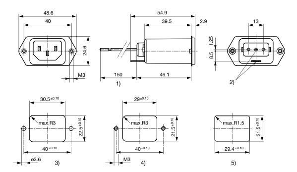
1) Flexible wire, standard length 150 mm or special length on request
