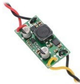
Pololu step-up/step-down voltage regulator S18V20x showing wires soldered directly to the board and passing through the
