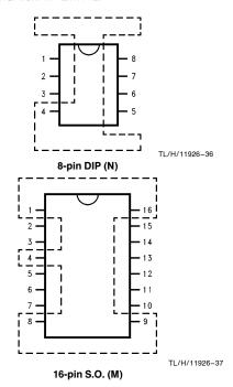
FIGURE 11. Copper Heatsink Layouts
