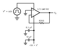
FIGURE 13. Start-Up Test Circuit
