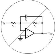
FIGURE 7. Compensation Capacitors Are Not Used with the LM6182, Instead Simply Increase R<sub>f</sub> to Compensate
