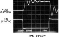
FIGURE 9A, 9B.  $A_V=-1$ , LM6182 Can Directly Drive 50 pF of Load Capacitance with 100 ns of Ringing Resulting in Pulse Response
