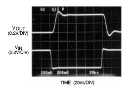
FIGURE 10A, 10B. Resistive Isolation of  $C_L$  Provides Higher Fidelity Pulse Response.  $R_f$  and Rs Could Also Be Increased to Maintain  $A_V=-1$  and Improve Pulse Response Characteristics.
